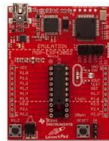
Figure 1: MSP 430 Launch Pad
